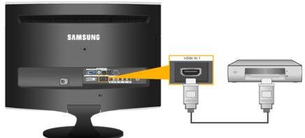
• Input devices such as digital DVD are connected to the *[HDMI IN 1]* terminal of the monitor using the HDMI cable. When all the connections are completed, connect the power cords for the monitor and DVD(or the device connected to the digital output terminal).
